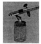
reservoir. Hold the front shell of the air brush firmly to attach or remove the paint jar to avoid unnecessary wear and tear on the rotary seal. Give the stem of the jar adapter a slight counter clockwise turn to snug the jar securely into place. To remove the jar when finished pull down and rotate in a clockwise direction.
