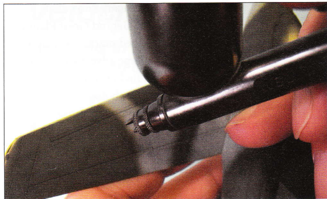
Holding the Velocity at a 45 degree angle produces a good-looking feathered edge to camouflage lines.
